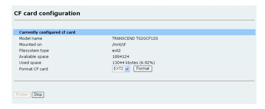
Figure 6-1 ATA/IDE fixed disk card configuration
