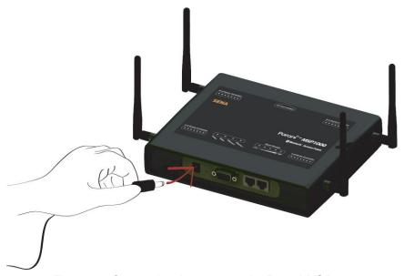
Figure 2-2 Connecting the power to the Parani-MSP1000
