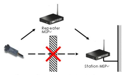
Figure 4- 2 Bluetooth communication using Repeater
