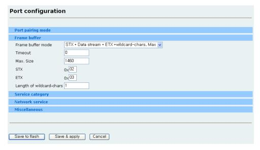
Figure 5-6 Frame buffer configuration
