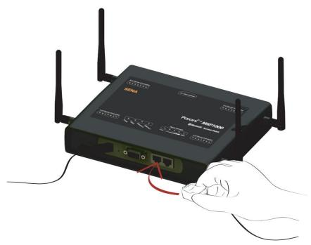
Figure 2-3 Connecting a network cable to the Parani-MSP1000
