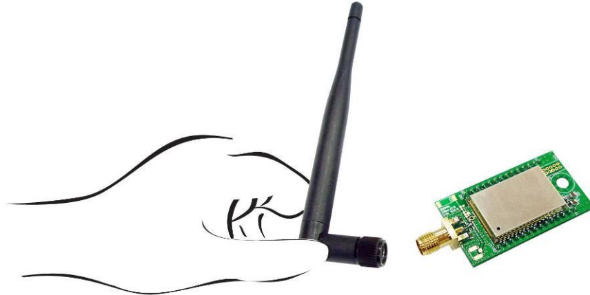
Figure 2-2 RP-SMA Dipole Antenna Installation
